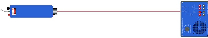
Figure 8. Class IIIa laser and laser beam aligned with an Industrial Fiber Optics' audio laser receiver for demodulation of the laser beam's modulated signal and producing sound waves.
