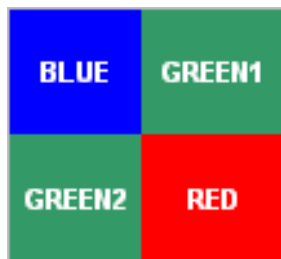
Figure 3. Color Filter Arrangement on the Pixels
