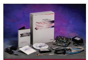
Embedded Development HW/SW Kit – Spartan-3A DSP S3D1800A MicroBlaze Processor Edition
