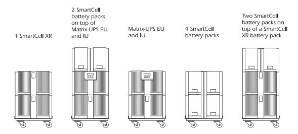
The Matrix-UPS cart will safely support any of the load configurations shown above. These are:
