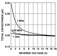
Figure 2. RF Capacitance vs. Reverse Bias.
