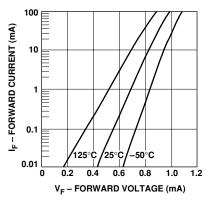
Figure 1. Forward Current vs. Forward Voltage.
