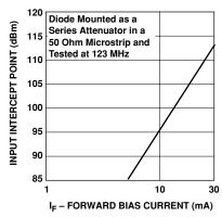
Figure 5. 2nd Harmonic Input Intercept Point vs. Forward Bias Current for Switches.
