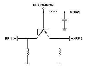
Figure 9. Switch Using Both Positive and Negative Current.
