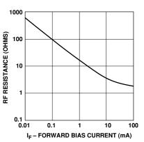
Figure 3. RF Resistance at  $25^{\circ}\mathrm{C}$  vs. Forward Bias Current.
