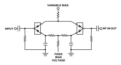
Figure 11. Four Diode  $\boldsymbol{\pi}$  Attenuator. See AN1048 for details.
