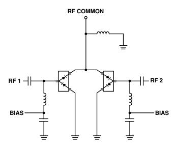
Figure 8. High Isolation SPDT Switch, Dual Bias.
