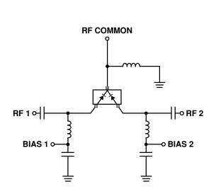
Figure 7. Simple SPDT Switch, Using Only Positive Current.
