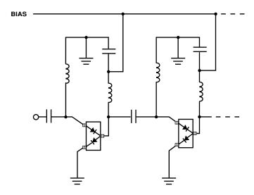
Figure 12. High Isolation SPST Switch (Repeat Cells as Required).
