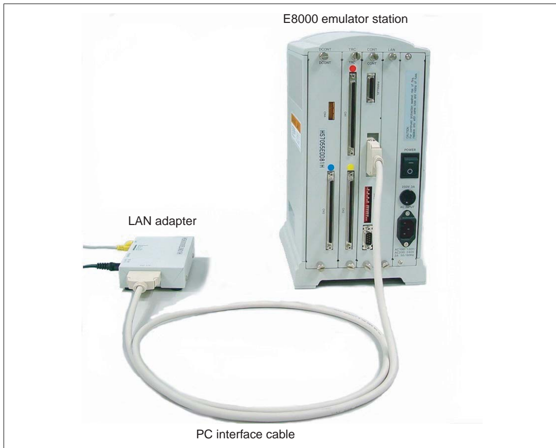
Figure 3.5 Connecting LAN Adapter to E8000 Emulator
