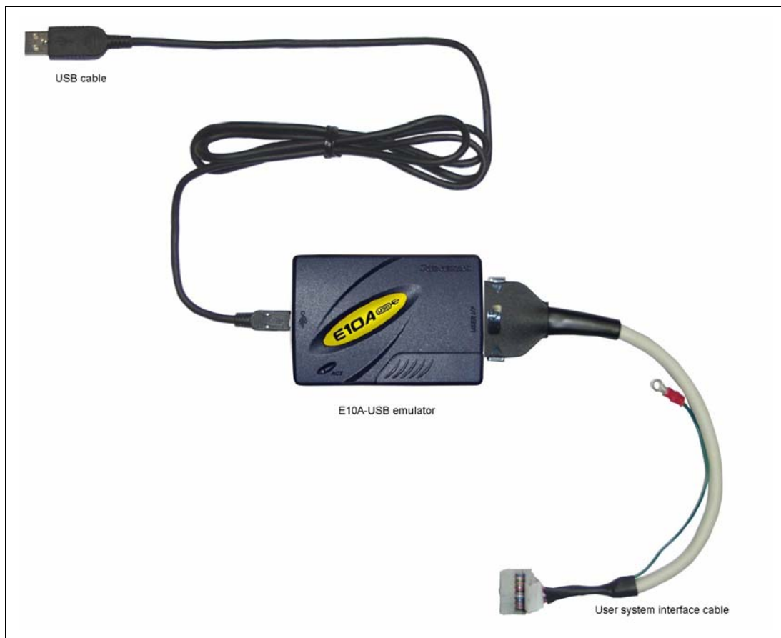
Figure 3.2 Emulator Hardware Configuration (when the 14-pin Type Connector is Used)
