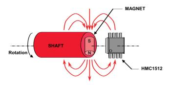
+/- 90 Degrees with a single HMC1512 Full 360 Degree Sensing with an Additional Hall Sensor
