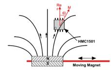
sors know the exact position and do not require indexing. Rare Earth magnets such as Neodymium or samarium cobalt types can be substituted with cost-effective Alnico or ceramic type magnets in typical applications such as linear displacement, angular displacement, motor control, and valve position.
