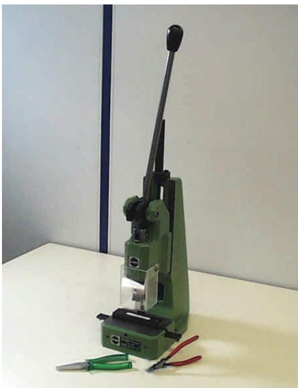
Figure 17 -- Connector Removal tooling HM2Y350
