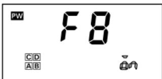
③ Press **WRITE** to confirm the setting. (The symbol on the sub-display will change from flashing to lighting.)
