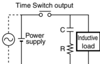
As a rough guide, the capacitor (C) and resistor (R) should have the following specifications:
