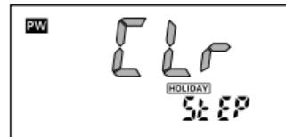
※ If **CLEAR** is pressed while "L Lr" is flashing, clearing operation is cancelled.
