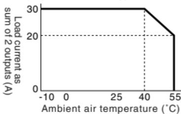
If wires with a temperature rating of 105 °C or higher are used, see the derating curve in the Section 4, "Ratings and characteristics".
