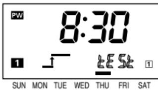
③ If **WRITE** is pressed while displaying the last setting for the week, "End" is displayed for 2 s and the Time Switch automatically returns to run mode.
