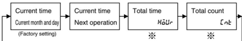
※ Displays only when the input selection is set to “**TL**”. (
