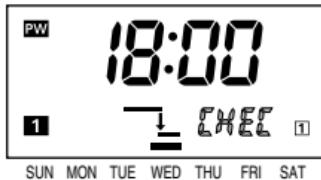
③ If **WRITE** is pressed with the last setting of the day displayed, “End” is displayed for 2 s before the Time Switch automatically returns to run mode.
