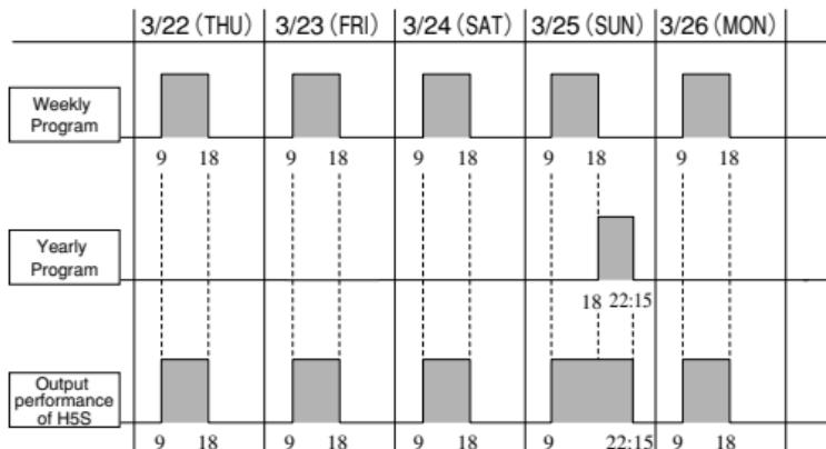
※If a weekly program and a yearly program overlap in operation time, the output of the H5S is continuously produced without being interrupted.
