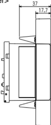
When mounting the H5S on exposure, always install the large terminal cover, Y92A-72H (separately purchased).
