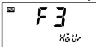
② Alarm value setting display appears automatically in 2 s after entering F3. Press **h** or **m** to set an alarm value. (Pressing **⊖** decrements the value of the Key that was last pressed.)
