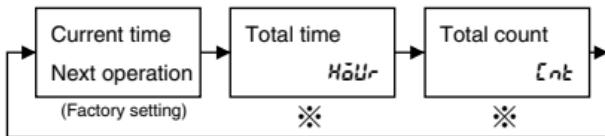
※ Displays only when the input selection is set to “**TL**”. (
