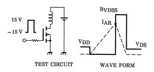
$$\begin{aligned} &R_G = 25~\Omega \\ &V_{DD} = 25~V,~L = 371~\mu H \end{aligned} \qquad EAS = \frac{1}{2} \cdot L \cdot I^2 \cdot \left( \frac{BVDSS}{BVDSS - VDD} \right) \end{aligned}$$
