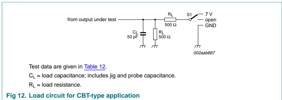
**Fig 12. Load circuit for CBT-type application**
