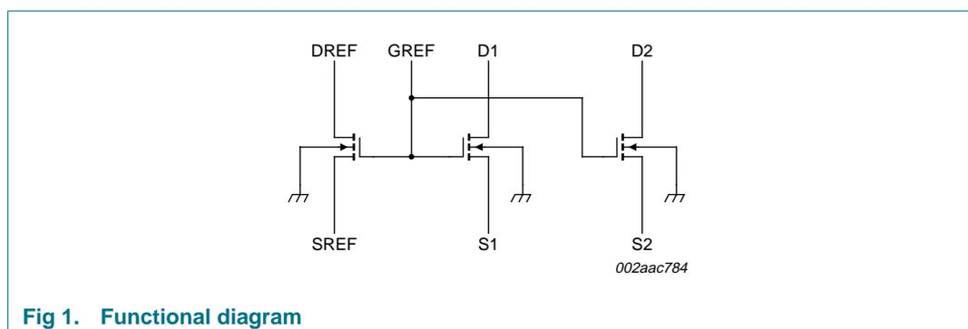
**Fig 1. Functional diagram**
