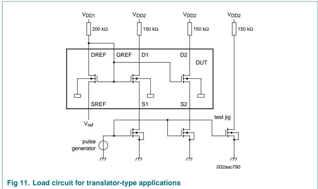
**Fig 11. Load circuit for translator-type applications**
