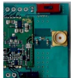
Figure 5. SMA connector for external antenna
