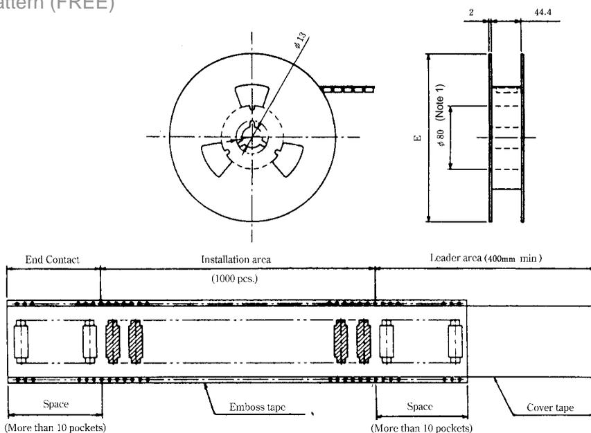
Note 1: E dimension for FX8C-140S-SV(92) is φ370, core dia. is φ100.
