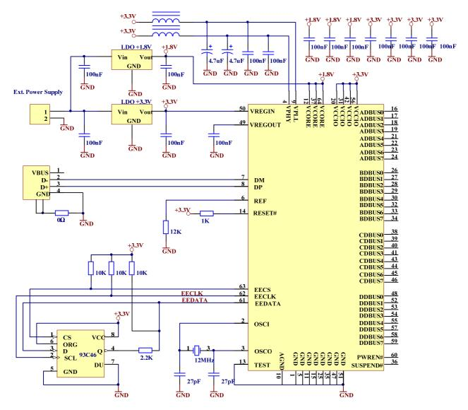
Figure 6.4 Self Powered Configuration Example 2
