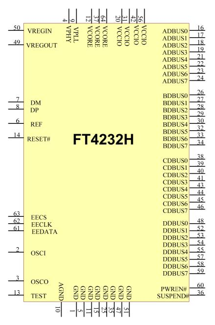
Figure 3.1 FT4232H Schematic Symbol
