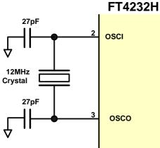
Figure 6.5 Recommended FT4232H Crystal Oscillator Configuration.
