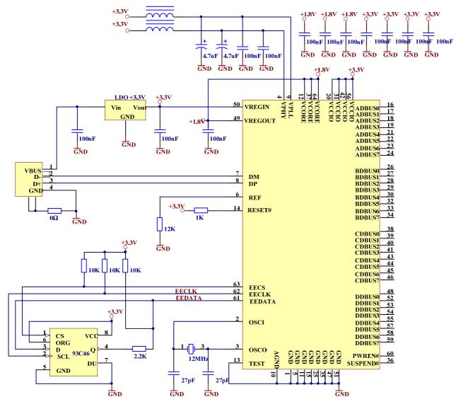
Figure 6.1 Bus Powered Configuration Example 1
