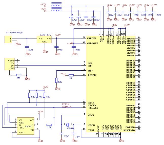
Figure 6.3 Self Powered Configuration Example 1
