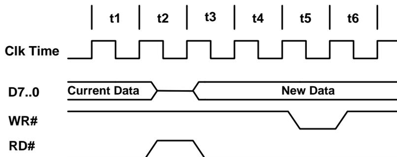
Figure 4.5 Synchronous Bit-Bang Mode Timing Interface Example
