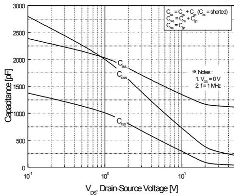
Figure 5. Capacitance Characteristics
