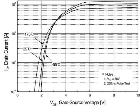
**Figure 2. Transfer Characteristics**
