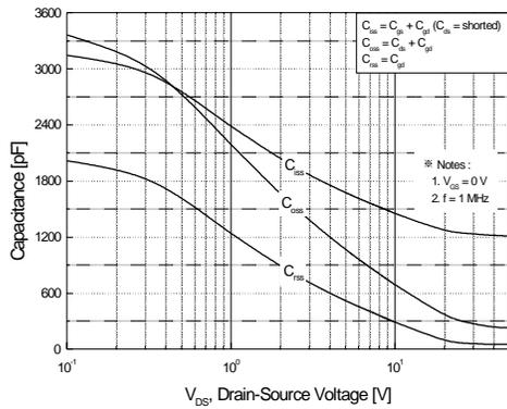
**Figure 5. Capacitance Characteristics**
