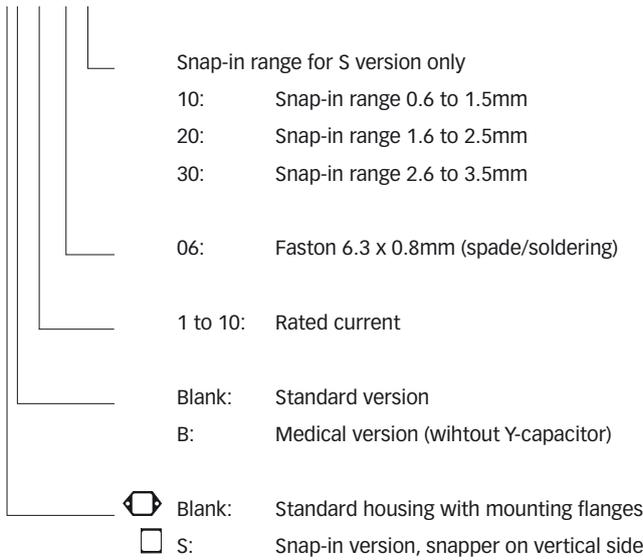
For example: FN 9260-1-06-10, FN 9260SB-10-06-20, FN 261S-6-06-30
