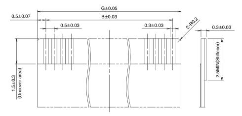
\*Polyimide and thermally hardening adhesive is recommended as the materials for the stiffener.
