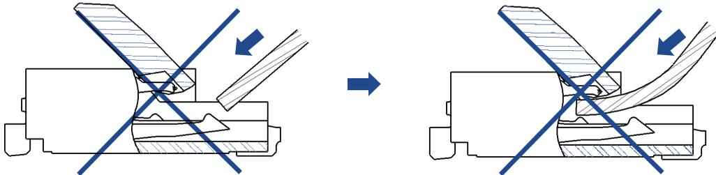
\*To avert insertion of the FPC on an angle, consideration should be given to securing FPC insertion space at the time of board layout. Insertion will be difficult when the FPC is too short.
