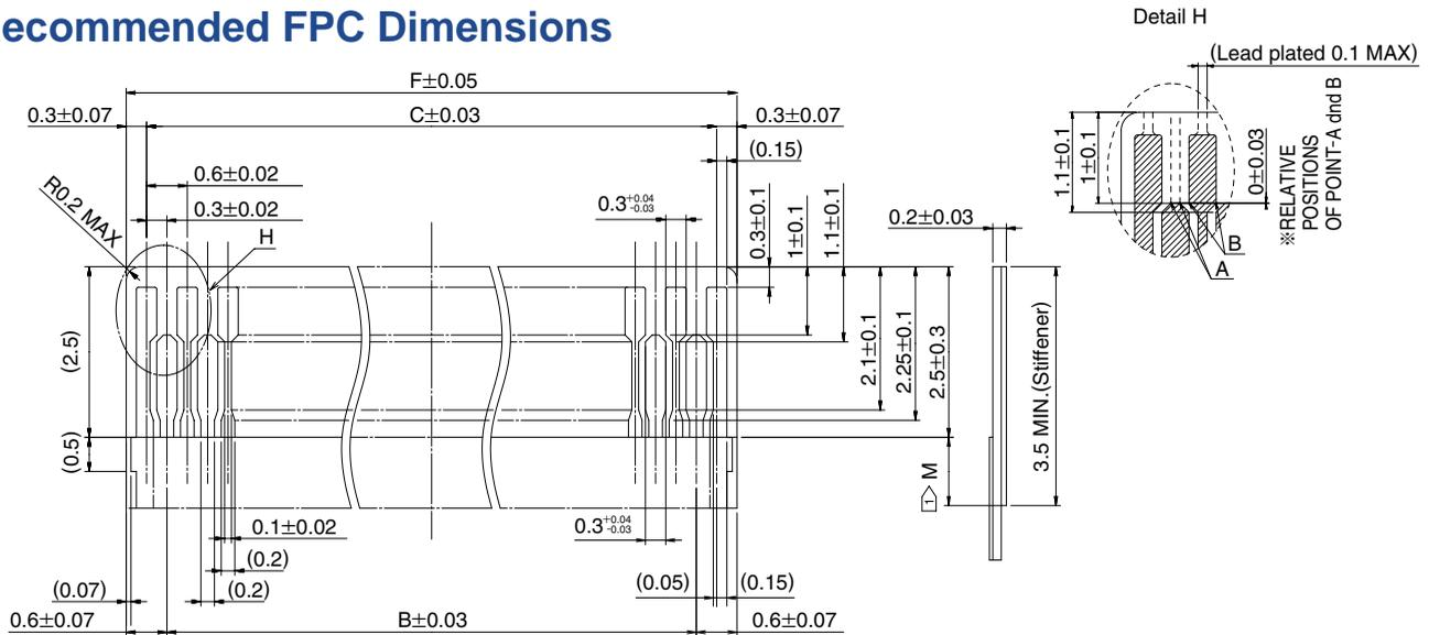
① Dimension M must be 0.5mm minimum when the stiffener is shorter than 3.5 min.
