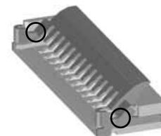
Actuator stays open during insertion of the FPC/FFC.
