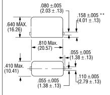
NOTE: FOR USE WITH TRACK MOUNT PER MIL-R-6106/23 \*\* MEASURED FROM SURFACE OF **HEADER**
