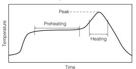
For soldering (Example: Sn/Pb)
