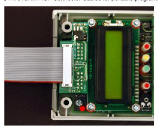
A special AT91SAM7 ISP cable has been developed which connects between an Equinox portable ISP programmer and any SAM7 Target System.
