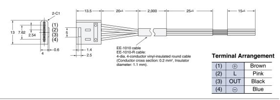
Applicable Photomicrosensors EE-SX67□ (A,P,R) (Connector Models only), EE-SX47□, EE-SY67□, EE-SPY31□/41□ EE-SPX303/403, EE-SPW311/411
