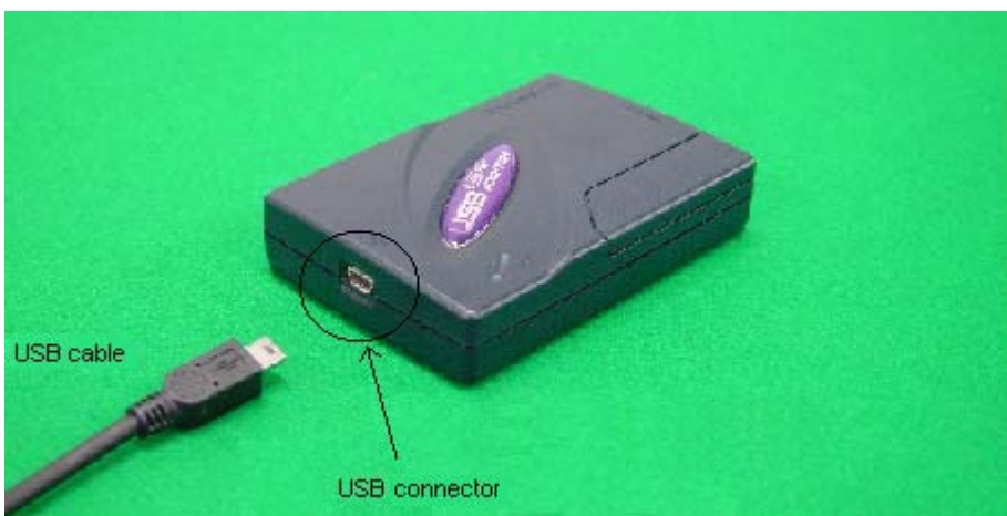
Figure 3.1 Connecting USB Cable to USB Adapter
