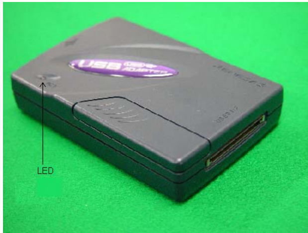
Figure 5.1 LED for Displaying the Communication State
