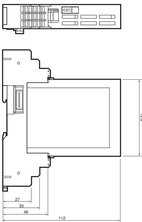
When mounting Units side-by-side, purchase the E5ZN-2□□□03□-FLK together with the E5ZN-SCT18S-500 for the second and subsequent Units.
