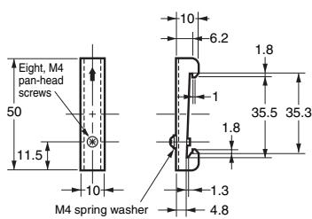
**Note:** End Plates are provided with the E5ZN-SCT24-500. Be sure to mount End Plates at both ends of Unit blocks.
