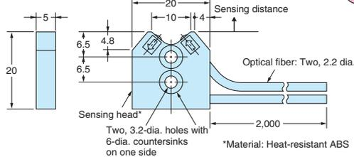
Note: There is a white line on the fiber that is inserted in the emitter-side port.
