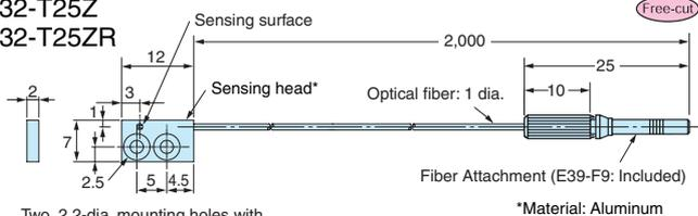
Two, 2.2-dia. mounting holes with two, 4.4-dia. countersinks on both sides
