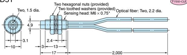
Note: The maximum allowable temperature is 150°C. The maximum allowable temperature for continuous operation is 130°C.
