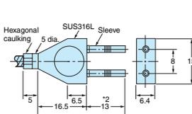
Note 1. The maximum allowable temperatures for sections A and B are 350°C and 110°C, respectively. The section inserted into the Amplifier Unit (indicated by \*2), however, must stay within the Amplifier Unit's operating temperature range.
