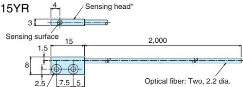
Two, 2.2-dia. mounting holes with two, 4.4-dia. countersinks on both sides
