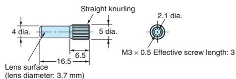
**Note:** This is the Lens Unit for the E32-C31 and E32-C41.
