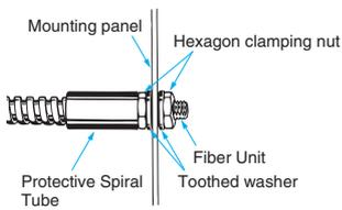
3. Secure the Protective Spiral Tube on a suitable place with the attached nut.
