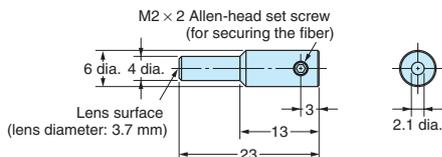
**Note:** This is the Lens Unit for the E32-D32 and E32-C42.
