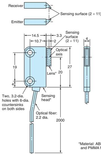
\*Material: ABS for the sensing head and PMMA for the lens.
