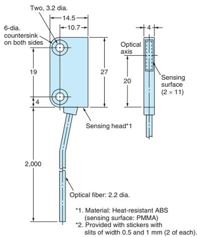
\*1. Material: Heat-resistant ABS (sensing surface: PMMA)
