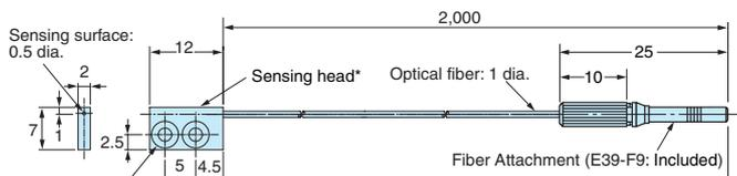
Two, 2.2-dia. mounting holes with two, 4.4-dia. countersinks on one side
