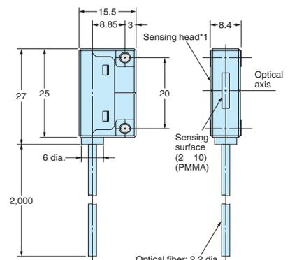
\*1. Material: Heat-resistant ABS (sensing surface: PMMA)
