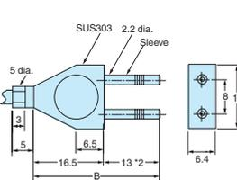
Note 1. The maximum allowable temperatures for sections A and B are 200°C and 110°C, respectively. The section inserted into the Amplifier Unit (indicated by \*2), however, must stay within the Amplifier Unit's operating temperature range.
