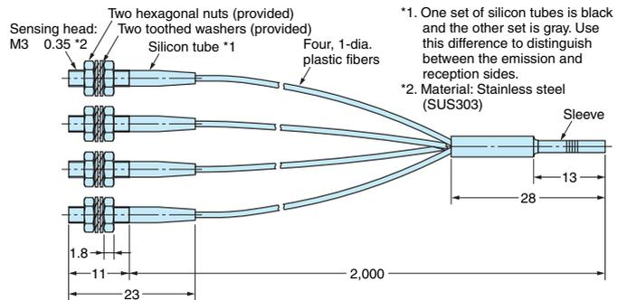
\*1. One set of silicon tubes is black and the other set is gray. Use this difference to distinguish between the emission and reception sides.
