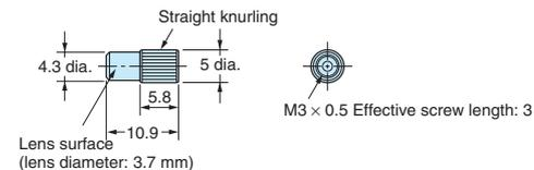
**Note:** This is the Lens Unit for the E32-C31 and E32-C41.
