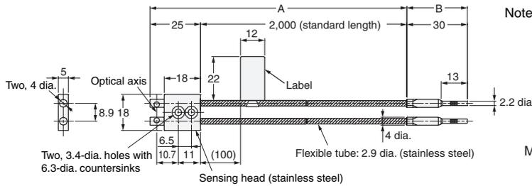
Note 1. The maximum allowable temperatures are 300°C for section A and 110°C for section B (section inserted into the Amplifier Unit).
