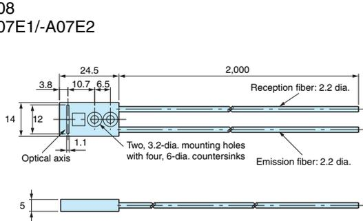
\* The E32-A07E1(E2) has a reception fiber and an emission fiber. Use the fiber with a model display tube (fiber with blue dotted line) as light emitting side.
