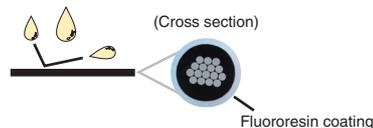
Fluororesin is used as the sheath material to prevent fiber degradation resulting from oil adhesion.
