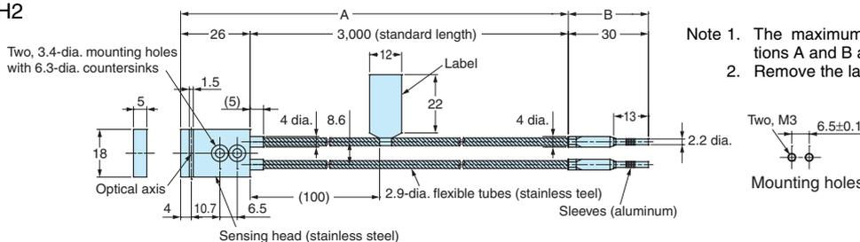
**Lens Unit for Reflective Fiber Units
