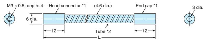
**Note 1.** The length L is 1,000 for the E39-F32A/-F32B and 500 for the E39-F32A5/-F32B5.
