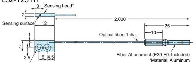
Two, 2.2-dia. mounting holes with two, 4.4-dia. countersinks on one sides
