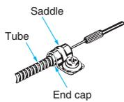
4. Use the attached saddle to secure the end cap of the Protective Spiral Tube. To secure the Protective Spiral Tube at a position other than the end cap, apply tape to the tube so that the portion
