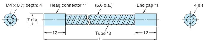
**Note:** The length L is 1,000 for the E39-F32C and 500 for the E39-F32C5.
