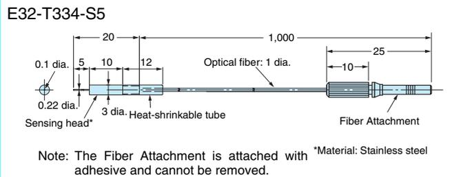
Special-beam Models **Fine-beam (narrow vision field) Models**
