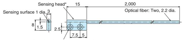
Two, 2.2-dia. mounting holes with two, 4.4-dia. countersinks on both sides
