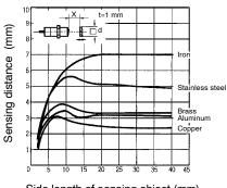
Side length of sensing object (mm)
