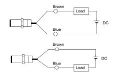
Note: It is possible to connect the load in two ways as shown in the above diagrams.
