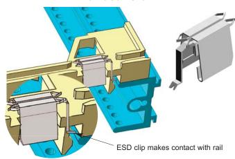
Electrostatic discharge clips (ESD) for VectorPak<sup>tm</sup> CG3-Series card guides will provide permanent ES discharge of the PCB before contact with connector
