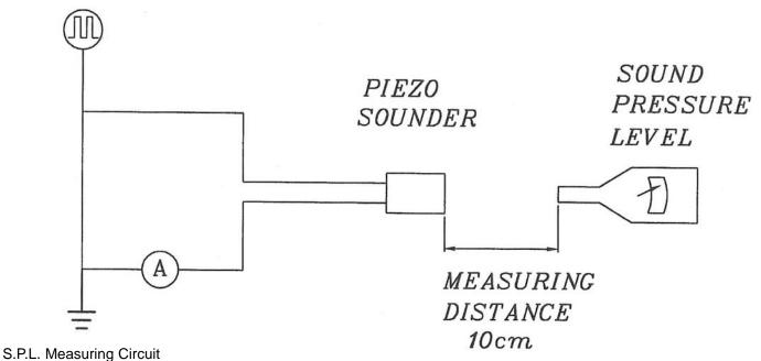
Input Signal: 10 V p-p, 4.0 KHz, Square Wave
