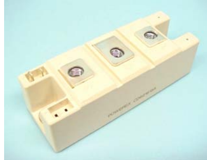
CD62__15B, CD67__15B Dual SCR/Diode Isolated POW-R-BLOK™ Module 150 Amperes / Up to 1800 Volts
