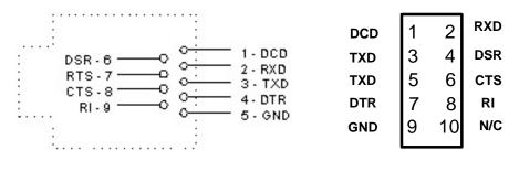
DB-9 Pin Out Top View 10 Pin Header Pin Out Top View
