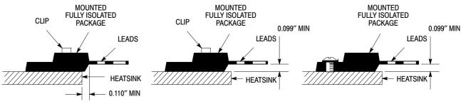
Figure 22a. Screw or Clip Mounting Position for Isolation Test Number 1
