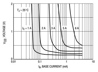
Figure 3. Collector Saturation Region
