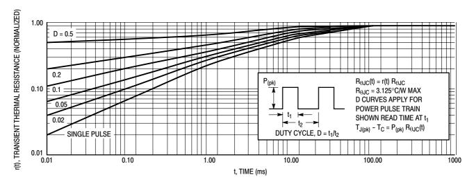
Figure 21. Typical Thermal Response for BUL146F
