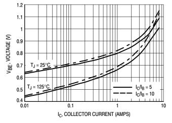
Figure 5. Base-Emitter Saturation Region
