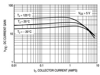
Figure 2. DC Current Gain @ 5 Volts
