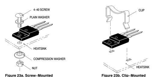
Figure 23. Typical Mounting Techniques for Isolated Package
