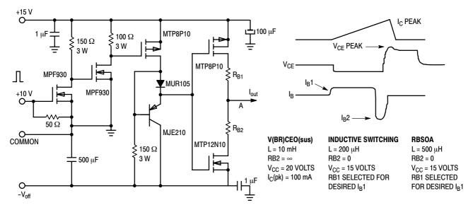
**Table 1. Inductive Load Switching Drive Circuit**
