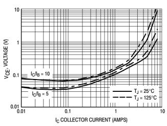
Figure 4. Collector-Emitter Saturation Voltage
