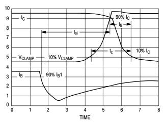
Figure 18. Dynamic Saturation Voltage Measurements
