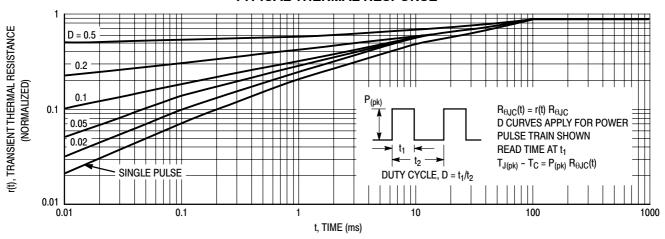
Figure 20. Typical Thermal Response ( $Z_{\theta JC}(t)$ ) for BUL146
