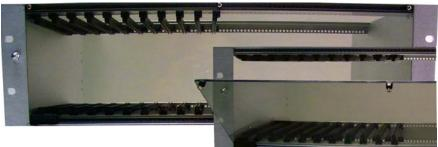
VectorPak<sup>IIII</sup> subrack hinged door panels screw directly into lower M2.5 tapped strip and secure at top M2.5 tapped strip with M2.5 captive screws. Doors can be added to any DIN subrack without exceeding 3U or 6U vertical height limitation. Aluminum doors are brushed aluminum with clear irridite finish. Polycarbonate doors are clear to light grey. Solid front or rear aluminum panels are 0.100"TH and attach to rack frame with M2.5 captive screws.
