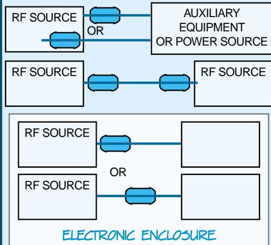
**POSITION OF SUPPRESSOR** The suppressor should normally be located close to the cable termination where it exits the enclosure. Where a cable connects two enclosures containing RF sources, a suppressor on each end may be required. For circuits within an enclosure, a position close to the RF is best. However, other locations along the circuit may work as well.
