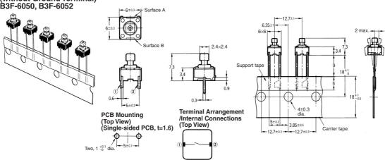
Note: The tape is random between surface A and surface B.
