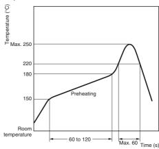
**Note:** The above heating curve applies if the PCB thickness is 1.6 mm.
