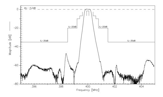
Transfer function (pass band, including losses of matching elements and balun):
