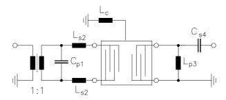
$$\begin{array}{ll} C_{p1} & = 4,7 pF \\ L_{s2} & = 39 nH \\ L_{c} & = 47 nH \\ L_{p3} & = 27 nH \\ C_{s4} & = 2,7 pF \end{array}$$
