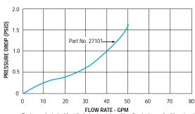
Tests conducted with units in horizontal position (lead wires up) with water at +70°F (21°C).
