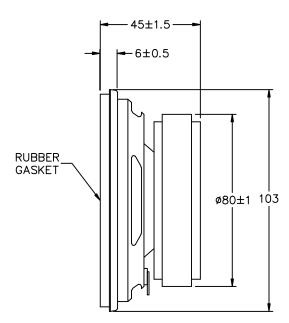
projects © unlimited UNLESS OTHERWISE SPECIFIED: DIMENSIONS ARE IN MILLIMETERS, TOLERANCES ARE ±0.5 AND ANGLES ARE ±3'. Dayton , Ohio SPEAKER DATE
