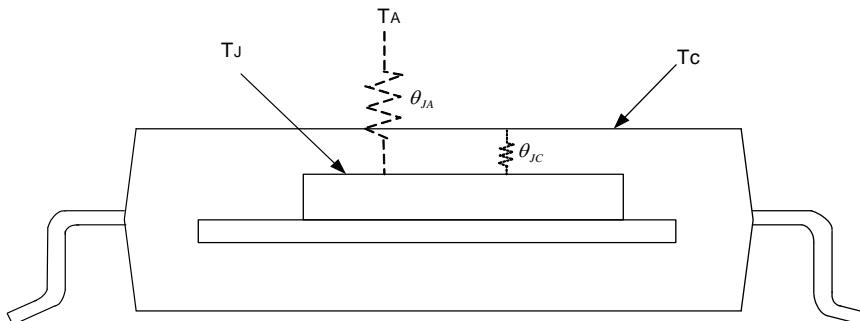
Notes: 3.  $\theta_{JA}$  should be confirmed with what heat sink thermal resistance. If no heat sink contacting,  $\theta_{JA}$  is almost the same as  $\theta_{JC}$ .
