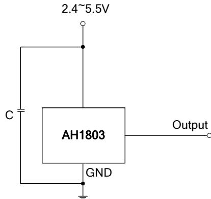
Notes: 4. C is for power stabilization and to strengthen the noise immunity, the recommended capacitance is 10nF~100nF.
