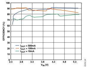
Figure 11. Efficiency vs. Input Voltage ( $V_{OUT} = 3.3 V$ )
