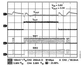
Figure 19. Load Transient ( $V_{IN} = 3.6 \text{ V } V_{OUT} = 3.3 \text{ V}$ ,  $I_{OUT} = 10 \text{ mA}$  to 300 mA)
