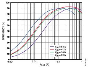
Figure 7. Efficiency vs. Output Current, PWM Mode (Vout = 3.3 V)
