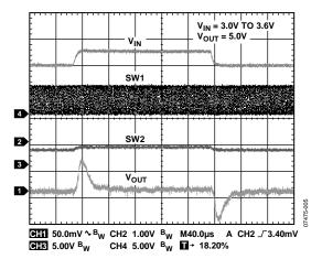
Figure 15. Line Transient, PWM Mode ( $V_{IN} = 3.0 \text{ V}$  to 3.6 V,  $V_{OUT} = 5.0 \text{ V}$ )
