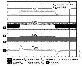
Figure 17. Line Transient, PWM Mode ( $V_{IN} = 3.0 \text{ V}$  to 3.6 V,  $V_{OUT} = 2.8 \text{ V}$ )
