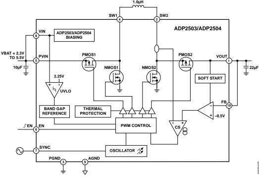
Figure 29. ADP2503/ADP2504 Block Diagram
