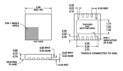
Figure 31. 10-Lead Lead Frame Chip Scale Package [LFCSP\_WD] 3 mm × 3 mm Body, Very Very Thin, Dual Lead (CP-10-9) Dimensions shown in millimeters
