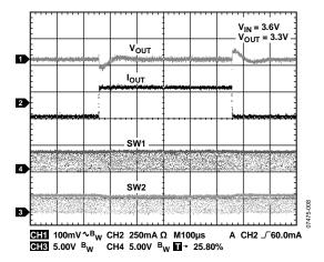
Figure 18. Load Transient ( $V_{IN} = 3.6 \text{ V } V_{OUT} = 3.3 \text{ V}$ ,  $I_{OUT} = 100 \text{ mA}$  to 350 mA)
