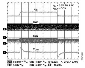
Figure 16. Line Transient, PWM Mode ( $V_{IN} = 3.0 \text{ V}$  to 3.6 V,  $V_{OUT} = 3.3 \text{ V}$ )
