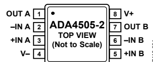
Figure 1. 8-Lead MSOP (RM-8)
