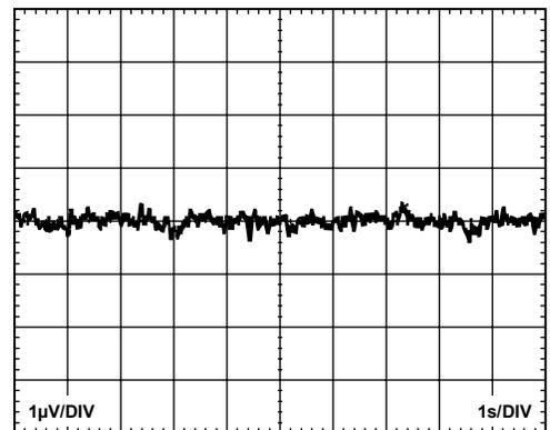
Figure 9. 0.1 Hz to 10 Hz RTI Voltage Noise ( $G = 1000$ )
