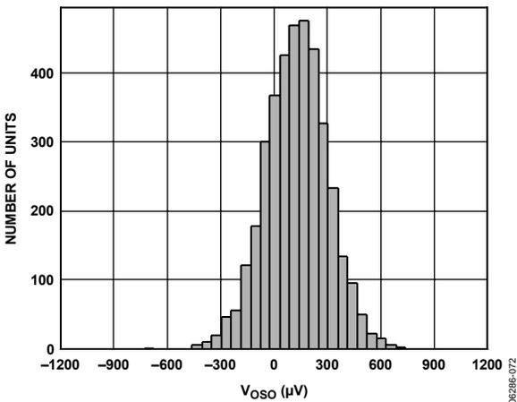
Figure 6. Typical Distribution of Output Offset Voltage
