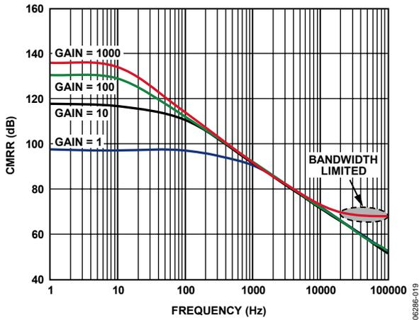
Figure 17. CMRR vs. Frequency, 1 kΩ Source Imbalance
