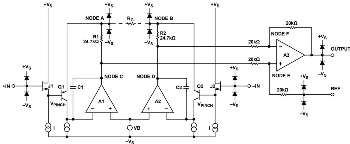
Figure 55. Simplified Schematic
