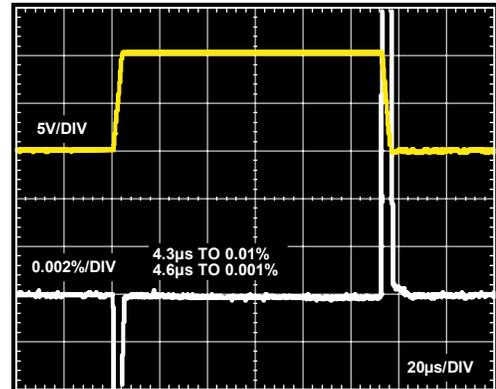
Figure 39. Large Signal Pulse Response and Settle Time,  $G = 10$ ,  $R_{LOAD} = 10\text{ k}\Omega$ ,  $V_S = \pm 15\text{ V}$ ,  $V_{REF} = 0\text{ V}$
