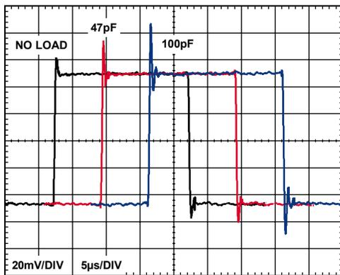
Figure 36. Small Signal Pulse Response for Various Capacitive Loads,  $V_S = 5\text{ V}$ ,  $V_{REF} = 2.5\text{ V}$
