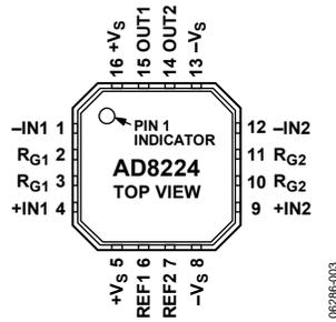
Figure 3. Pin Configuration
