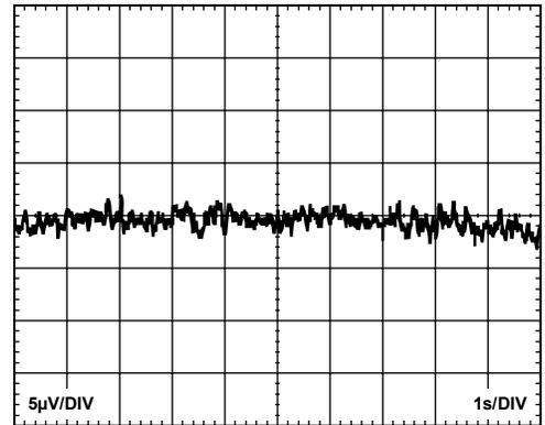
Figure 8. 0.1 Hz to 10 Hz RTI Voltage Noise ( $G = 1$ )
