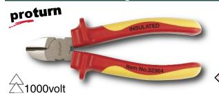
323 Proturn Insulated Diagonal Cutters. Insulation According to VDE 0682/part 201, DIN 7437, EN/IEC 60900, ASTM F-1505-01, NFPA70E, 1000 volt rated. Individually Tested. DIN ISO 5745 Pliers drop-forged from special tool steel, individually high frequency induction hardened, chrome and nickel plated, mirror polished. Proturn ergo soft grip handles for maximum comfort.
