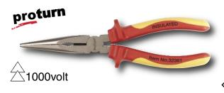
323 Proturn Insulated Long Nose Pliers. Insulation According to VDE 0682/part 201, DIN 7437, EN/IEC 60900, ASTM F-1505-01, NFPA70E, 1000 volt rated. Individually Tested. DIN ISO 5745 Pliers drop-forged from special tool steel, individually high frequency induction hardened, chrome and nickel plated, mirror polished. Proturn ergo soft grip handles for maximum comfort.
