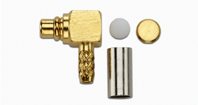
Model 73026 MMCX PLUG R/A CRIMP, RG178
