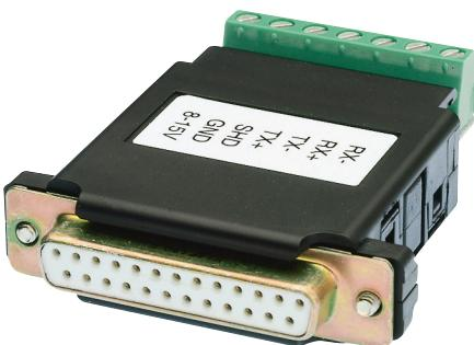
72-CNV-4 and 72-CNV-5 convert serial communications from RS-232 to RS-485 in both directions. The converter simply plugs into any male RS-232 DB-25 connector and converts the transmit and receive signals to RS-485 (RS-422) levels at speeds to 115.2 KB. The converters are configured for DTE (default) or DCE operation.
