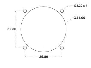
The joystick is dropped into the panel cut-out. For panel thickness of <3mm, M3 x 16 countersunk machine screws are recommended.
