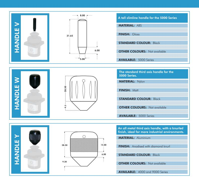
The total throw of all third axis handles is  $55^{\circ}$  (+/- 27.5 degrees). As standard the polarity of all the handles is incrementing when turned clockwise.
